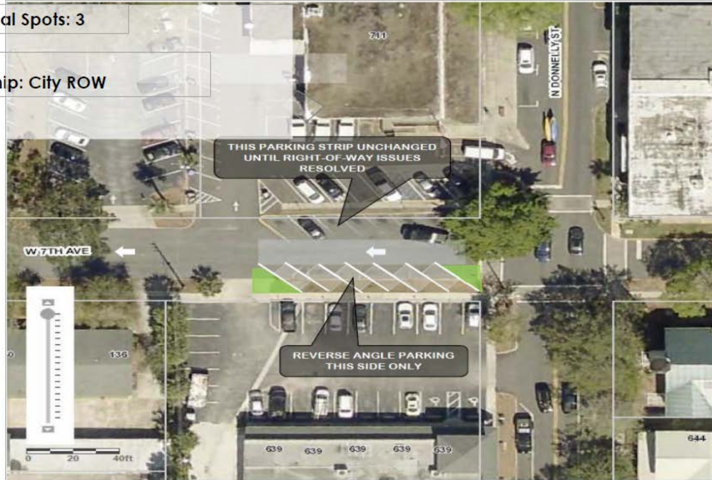
Reverse Angle Parking Scheme on South Side Only of W. 7 th Avenue between N. Alexander St. and N. Donnelly St. Six 9-foot wide by 16-foot long compact parking spaces (25-foot long stripe)
