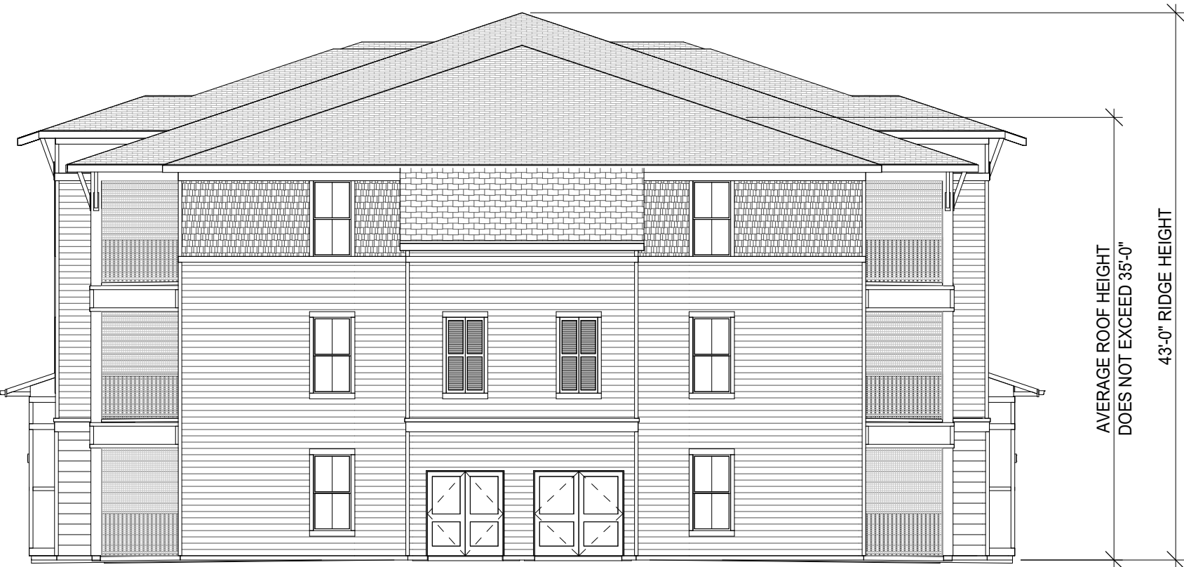
2 Building Type IV - Right / Left Elevation
