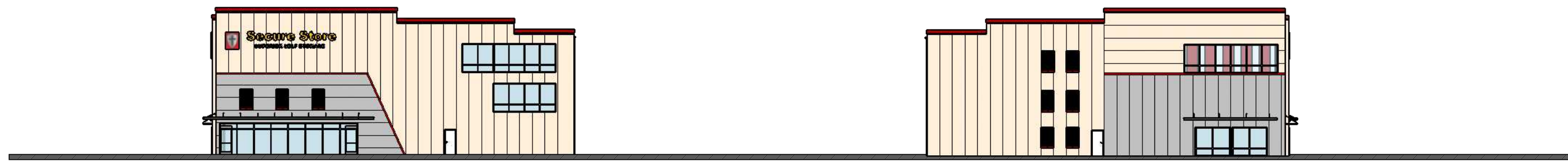
NORTH ELEVATION Windows/Shutters Actual 37% (Required 25%)
