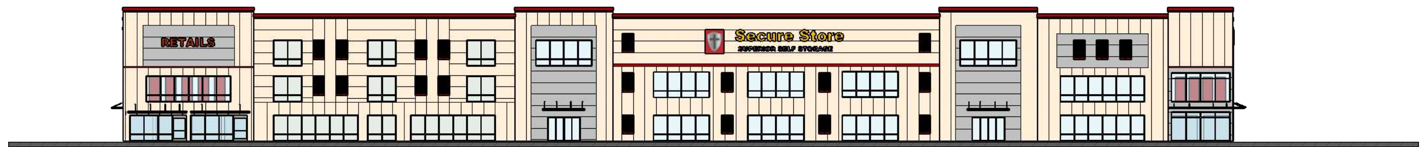
EAST ELEVATION Windows/Shutters Actual 40% (Required 40%)
